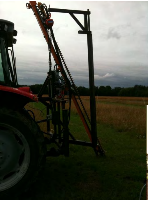
Drilling equipment for insertion of 3 m long minirhizotrons
